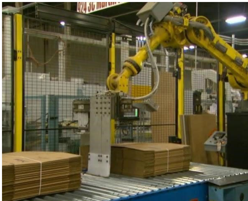
Exhibit 6. The Use of Robots to Handle Stacks of Cardboard
